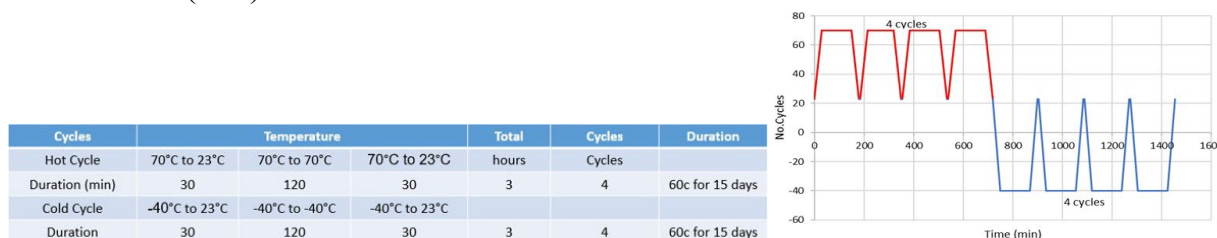
Figure 1: Test protocol details (left) and diagram (right) of OSB and plywood
