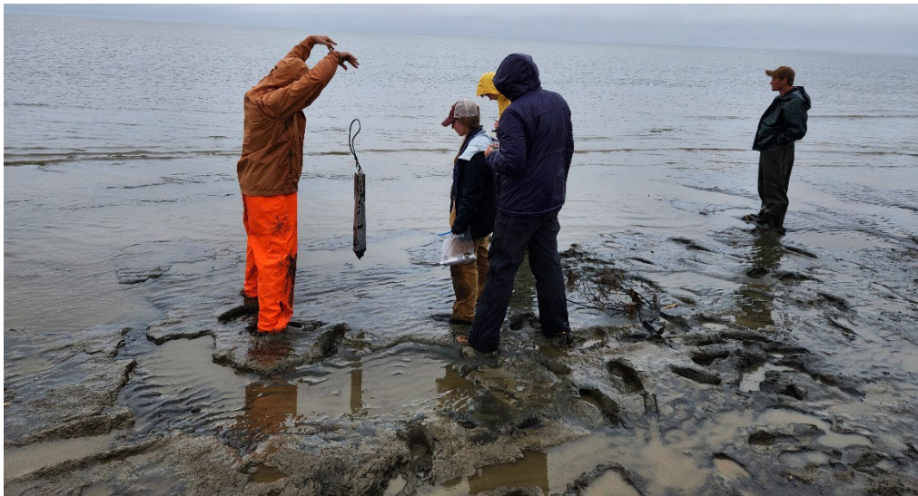
Fig. 2. PFFP deployment at the beach and intertidal zone in Quinhagak, AK in June 2022.
